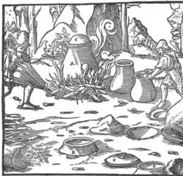
Fig. 16. Smelting bitumen from bituminous rocks "Destillatio per descensem" (after Agricola, De re metallica , 1556).
