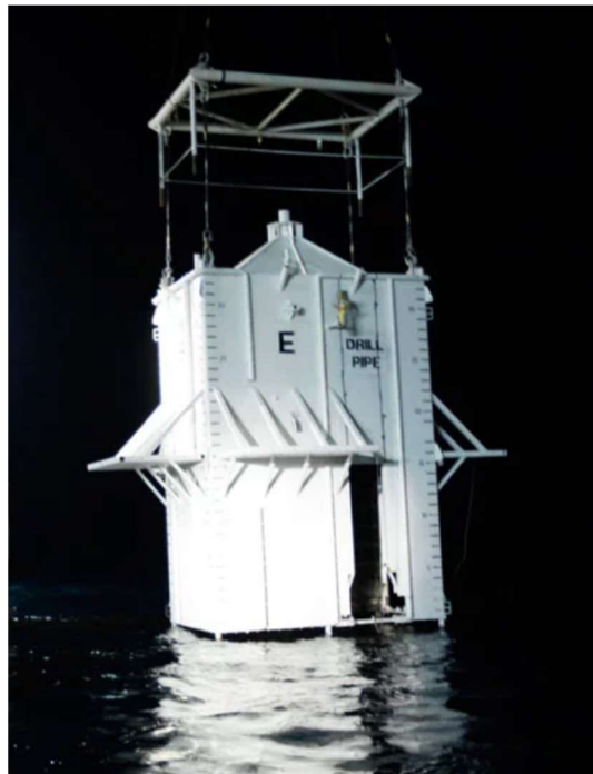
Photo 12: Oil containment dome used by Wild Well Control at BP Deepwater Horizon disaster - Macondo well 2010. Source internet images.
