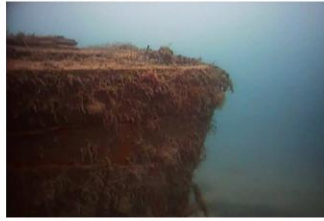
Underwater image of Bow of Investigator showing Hawsehole (opening for anchor chain)
